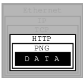
Figure 2. Sockets Covered Protocol Layers
